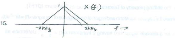
Consider the continous time band-limited signal x(t) with a spectrum x(f) as shown in figure above. Sketch the spectrum of the discrete signals x<sub>1</sub>[n] and x<sub>2</sub>[n] obtained from x(t) by sampling at 5 KHz and 3 KHz respectively.
